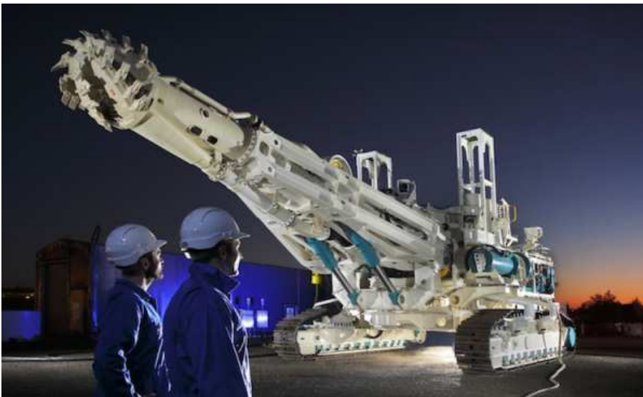
The Collecting Machine gathers cut material by drawing it in as seawater slurry with internal pumps and pushing it through a flexible pipe to the riser and lifting system
