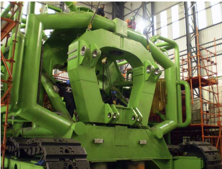
Mafuta, a new bottom-crawling diamond suction miner in 2013 when it was being built for De Beers, the diamond mining conglomerate. Photo via De Beers.
