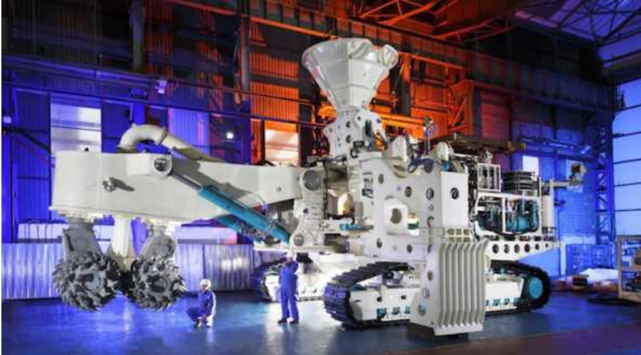
An Auxiliary Cutter goes along the sea floor first, removing rough terrain and creating benches for the other machines to work on. It has a boom-mounted cutting head for flexibility
