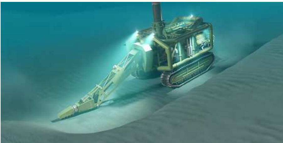
Trans-Tasman Resources proposes to use an undersea crawler to suck up iron-sand from the seabed. Graphic/ supplied
