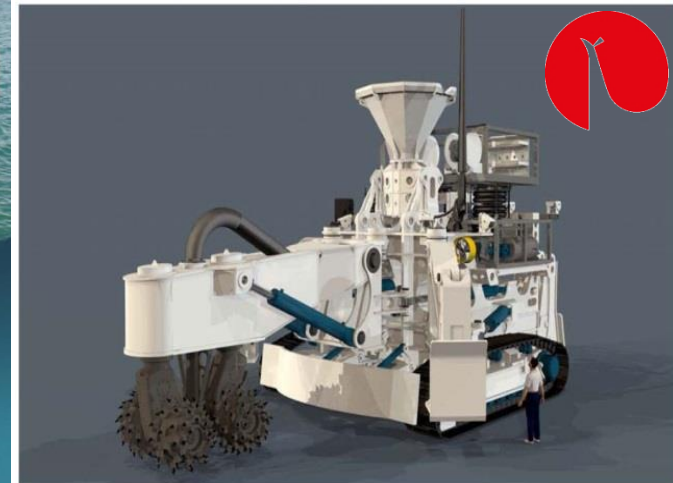
Auxiliary Cutter (AC) - cuts material on uneven surfaces, benching the site
