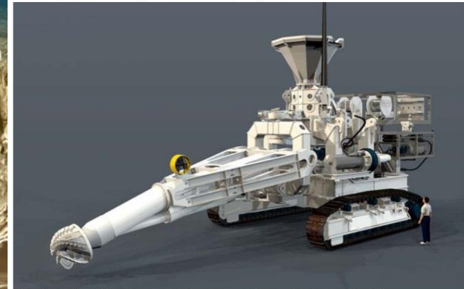
Collecting Machine (CM) - collects cut material with seawater, pumping and transfers the slurry to the RALS
