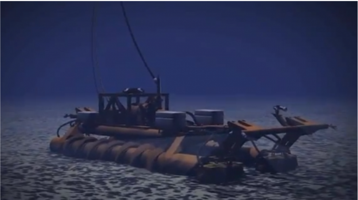
This computer generated image from Lockheed Martin suggests how the company could mine manganese nodules from the sea floor, using underwater vehicles that vacuum up nodules and transport them to a ship on the ocean surface. (Source: Lockheed Martin)
