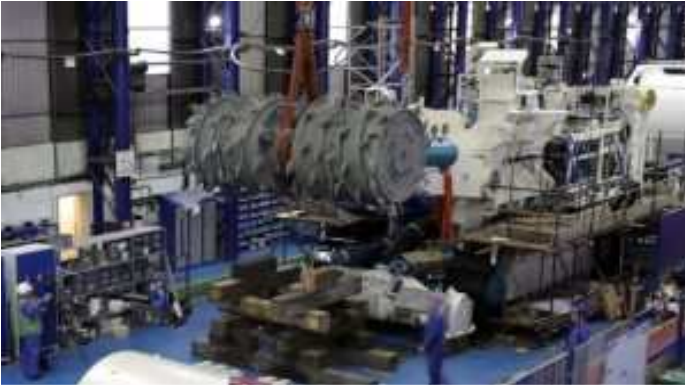
Construction of the largest machine - the 310-tonne Bulk Cutter
